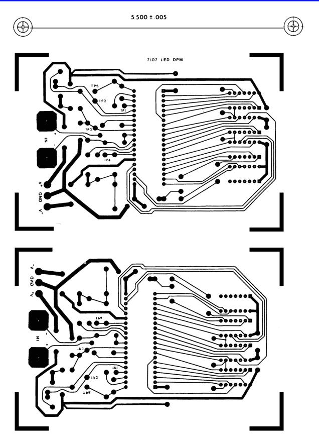
FIGURE 11. ICL7107 PRINTED CIRCUIT BOARD AND COMPONENT PLACEMENT
