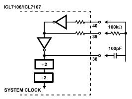
FIGURE 6. ICL7106/ICL7107 INTERNAL OSCILLATOR CLOCK
