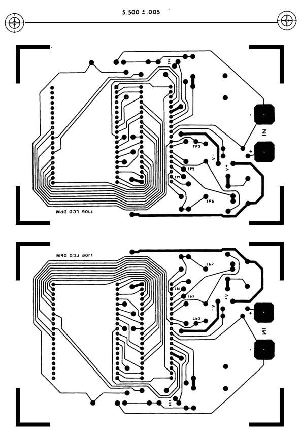
FIGURE 10. ICL7107 PRINTED CIRCUIT BOARD AND COMPONENT PLACEMENT
