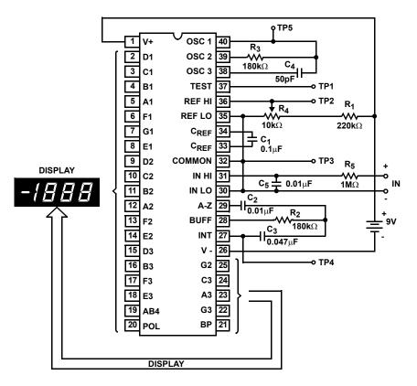
FIGURE 3. LCD DIGITAL PANEL METER USING ICL7136
